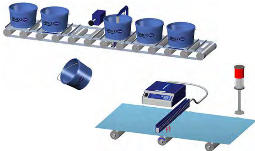
Detecting perforations in products
