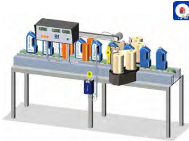
A Anti-static bar with airknife
