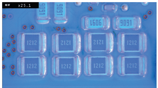
Complete coverage after Openair-Plasma® activation
