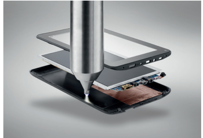
Plasma activation for quality-assured screen bonding
