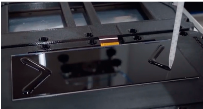
Application of LOCA to a plasma-activated glass surface.
