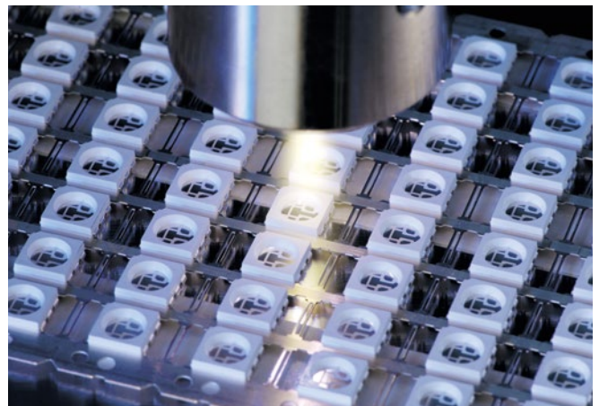
Application of the PlasmaPlus® layer on an 5050 type LED-leadframe
