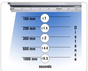
$\mu$ Wire AeroBar Model 5710 with 50mm Air Jet Spacing. Measured using Simco-Ion CPM Model 280A w/ HEPA flow (60 fpm or 0.3m/sec) & CDA flow at 50 lpm.
